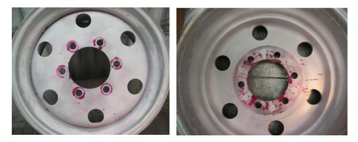
After 1.8 Million cycles radial fatigue - no cracks
