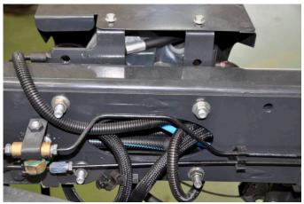
Rebolt to the chassis rail using the original bolts.
