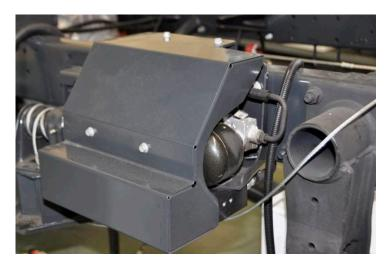
This is the differential box mounted on to the left hand chassis rail above the spare tire carrier.
